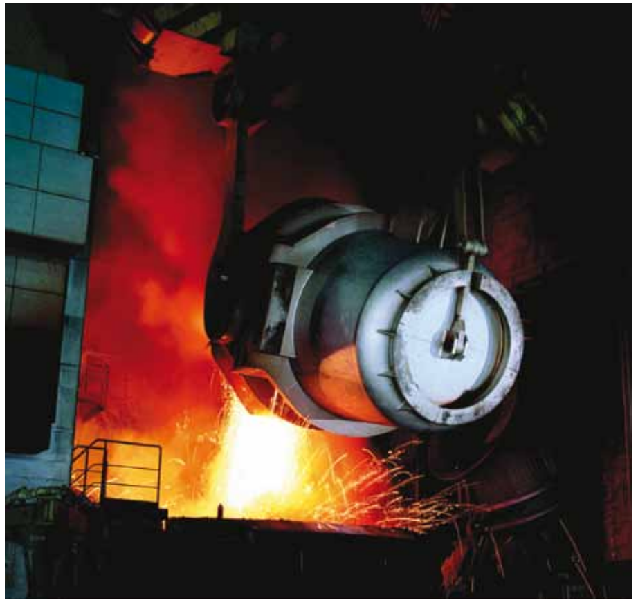
Batching liquefied steel in an electric furnace
