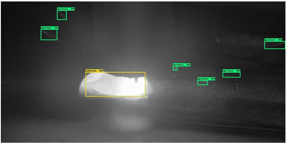
Figure 4: Example of real-time spatter (green) and weld pool (yellow) recognition using faster RCNN [source: Gestalt Robotics]
